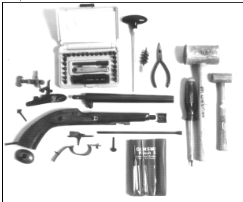
Figure 2, above. A disassembled percussion-lock, muzzle-loading "Brown Bess"-type pistol, showing the components and standard tools used in the conservation treatment of firearms.
